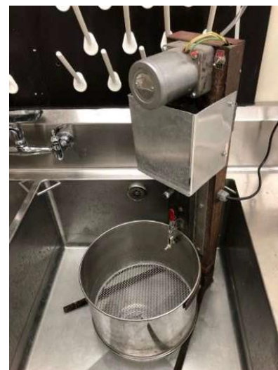
The wet sieving unit developed by CVAS. The unit moves the sieve up and down in water approximately 60 times per minutes to wash particles through the 4.75 mm sieve aperture.
